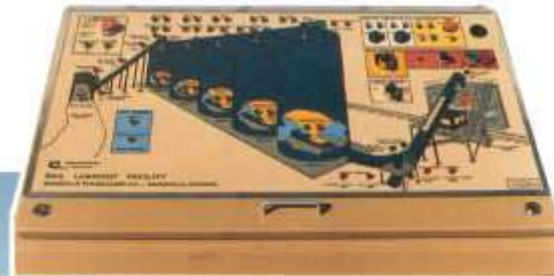
System control panel with graphic display and indicator lights for each component, allow one-man operation of the complete terminal.
